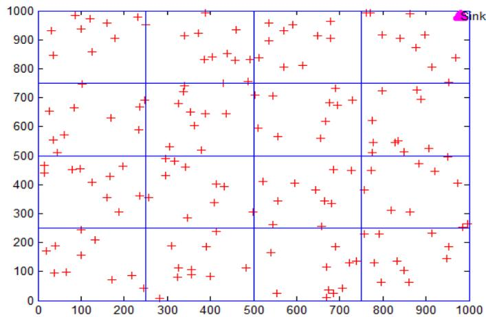
3. Each cluster will have one cluster head because instead of harvesting all energies of the node, Cluster head will communicate on behalf of each cluster for the conservation of energy and it will communicate with the sink node.
