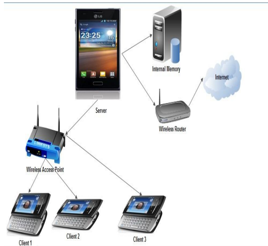
Figure 5.1: System Architecture of M-VLAN
