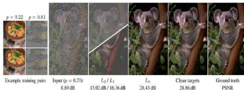
Figure 6 : For random impulse noise, the approx. mode-seeking L0 loss performs better than the mean (L2) or median (L1) seeking losses.
